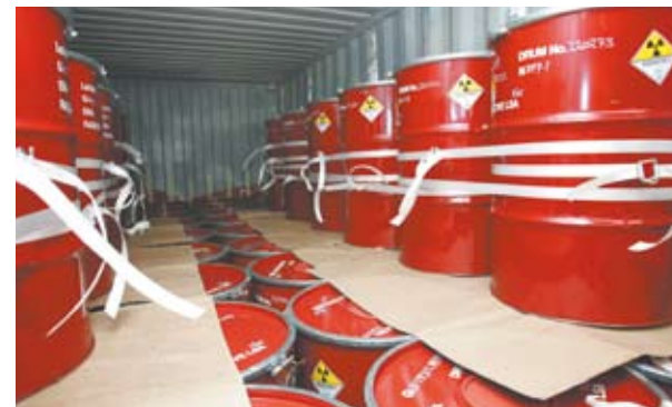
Packed container showing securing of top row of drums.
